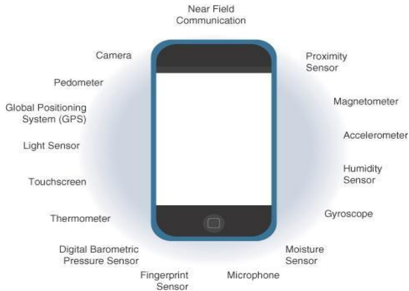
Figure 2.1: Sensors in a smart phone
